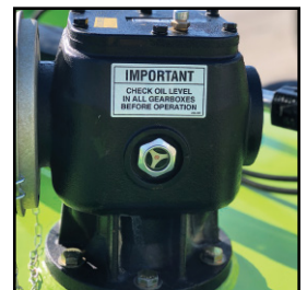
Convenient oil level site glass on gearboxes
