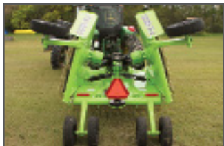
Narrow transport over-centering wing design
