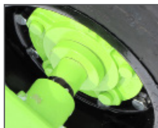
Metal seal guards on 517 hubs
