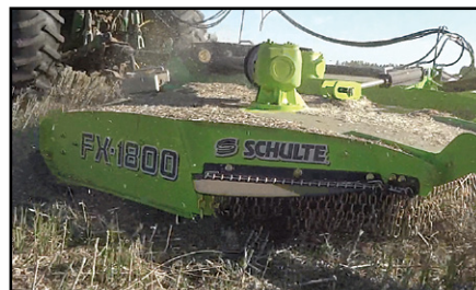
Outboard blade rotation on fixed knife model keeps material from balling up under the deck
