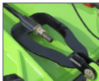
Single levelling rod with floating hitch
