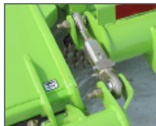
Greaseable adjustable turnbuckles for parallel levelling
