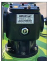
Convenient oil level site glass on gearboxes
