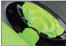
Metal seal guards on 517 hubs
