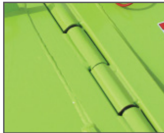
Heavy duty cast hinge line with wiper seals
