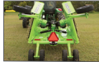
Narrow transport over-centering wing design
