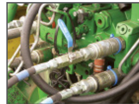
Ball valve wing lock up system
