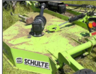
Continuously welded single domed deck
