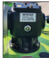
Oil level site glass on gearboxes
